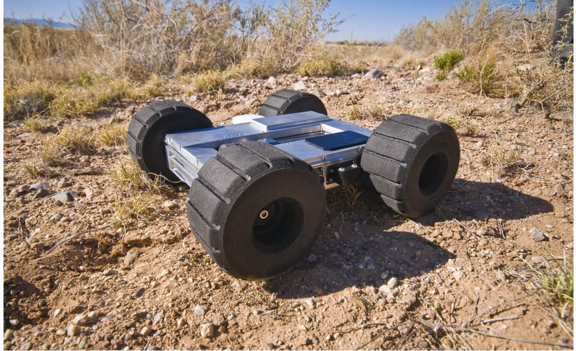
A hopping robot made to jump great heights. This robot utilizes a fairly basic wheeled chassis.
