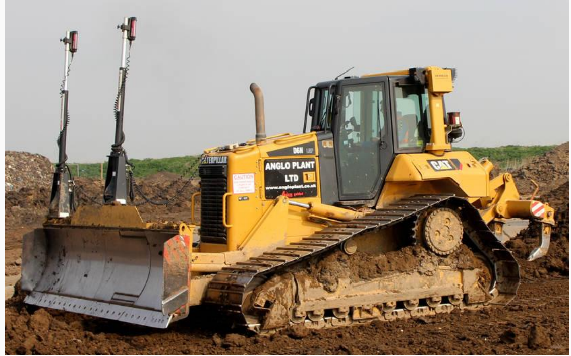
A bulldozer is a great example of a vehicle with a tracked chassis.
